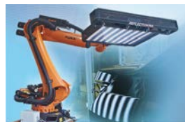
Deflectometry systems for automatic inspection of shiny surfaces reflectCONTROL Page 12-13
