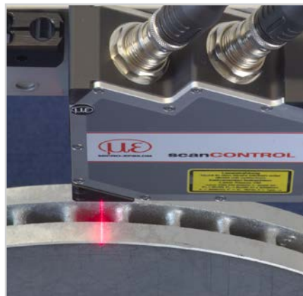
Profile measurements on brake disks
