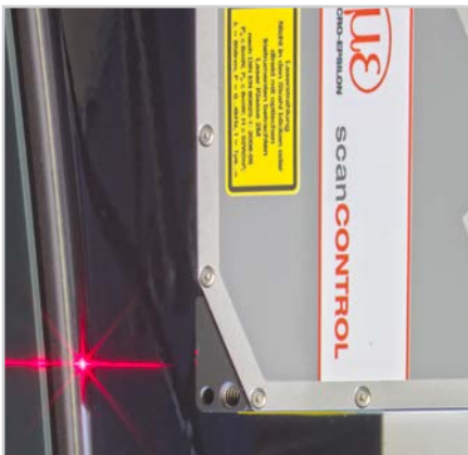
Gap measurement on a car body
