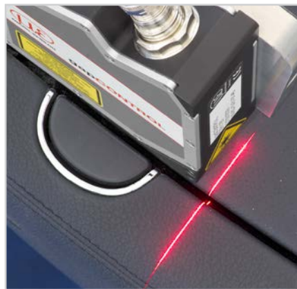
Distance measurement at the centre console
