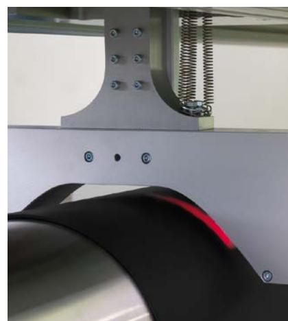
Thickness measurement of flat plastic film and rubber strips
