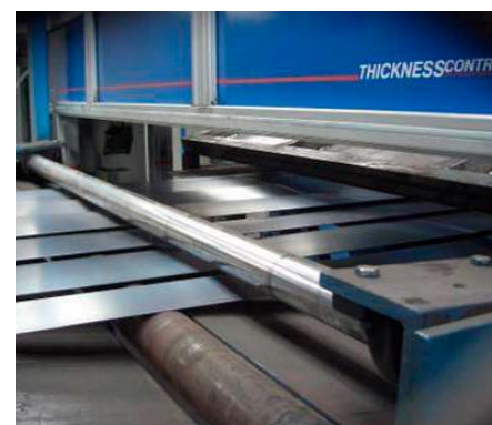
Measurement after slitting shears
