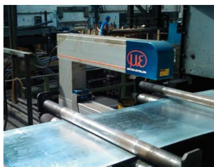
Thickness measurement in a forming line
