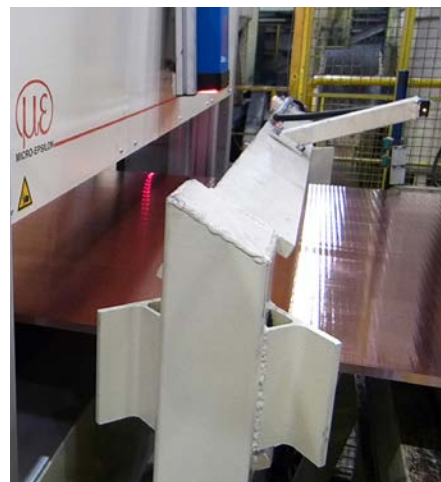
Thickness measurement in a milling line
