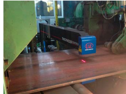
Thickness measurement in a milling line
