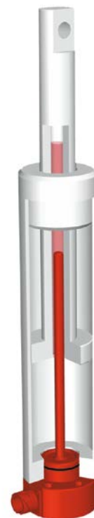
EDS series: integration in a hydraulic cylinder
